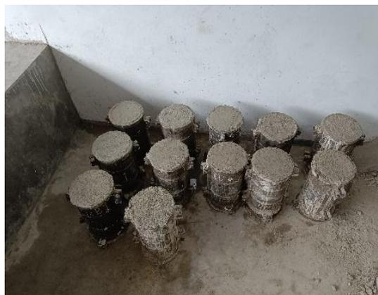
**Gambar 1.** Benda uji beton beton silinder  $F_c$  25 Mpa
