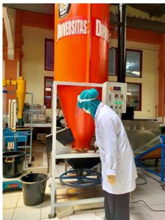
Gambar 1. Unit pengering vertikal model screw
