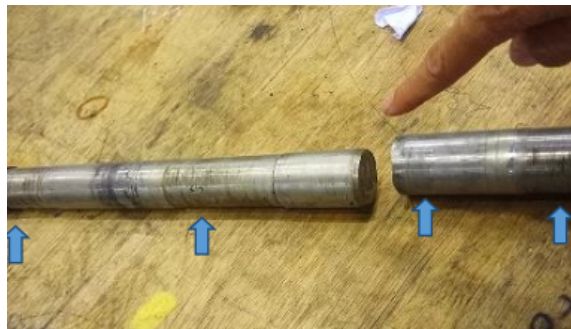
Figure 4. Shaft cross section area reduction caused by wearing out of bearing bushing
