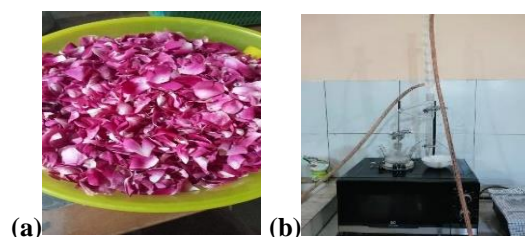
Figure 1. (a). Rose flower sample (b). MAHD Apparatus
