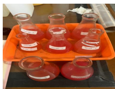
Figure 6. Titration Results of Papaya Seed Oil for Determination of FFA Levels
