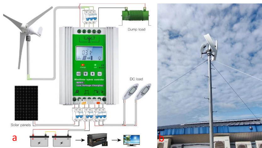
Figure 4. Pilot hybrid solar-wind power, (a) schematic, (b) wind turbine
