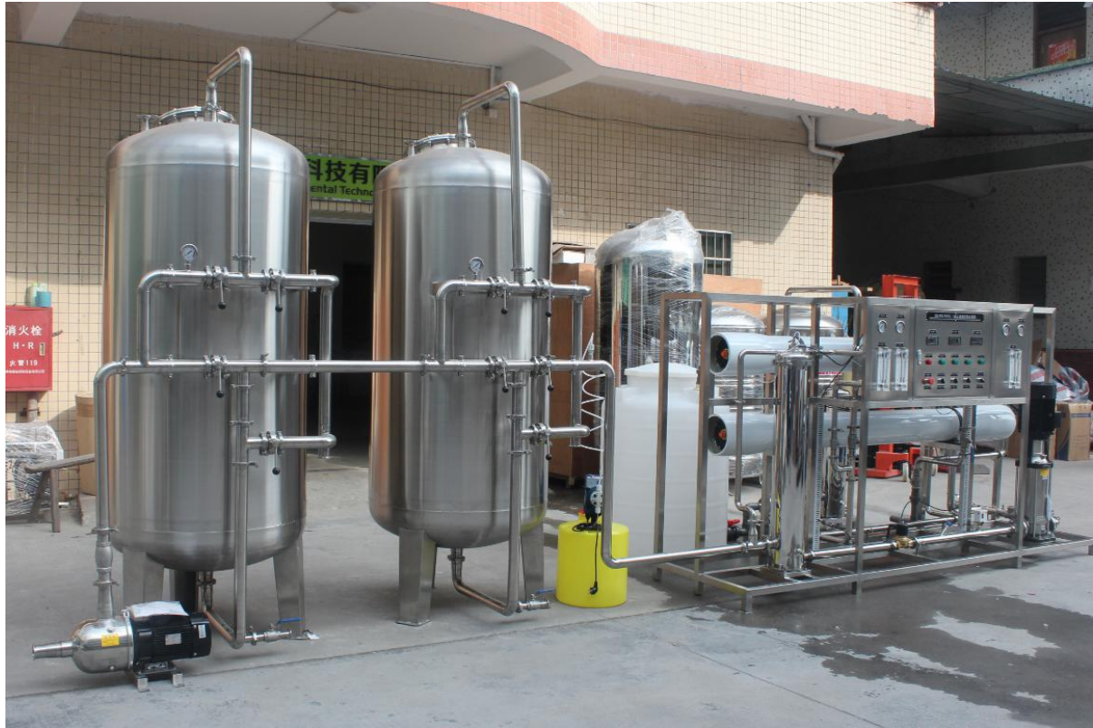
Figure 2. Proposed water treatment plant for ESPOCH
