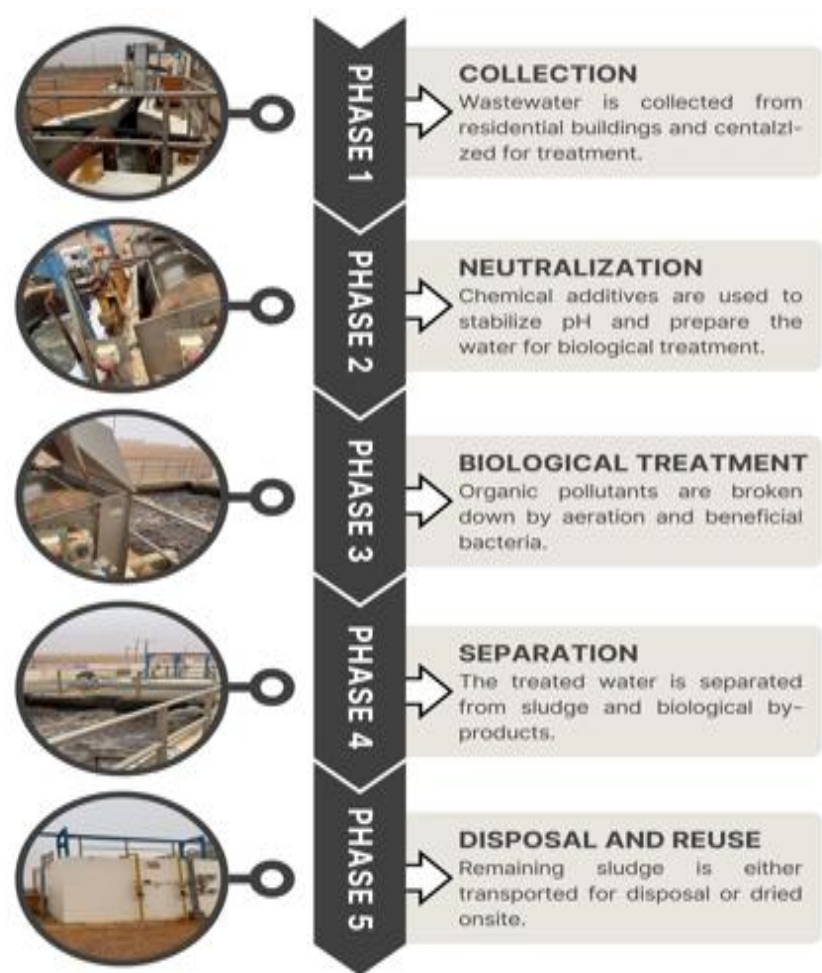
Figure 4. Five-stage wastewater treatment process at Shaqra University, covering collection, neutralization, biological treatment, separation, and reuse.
