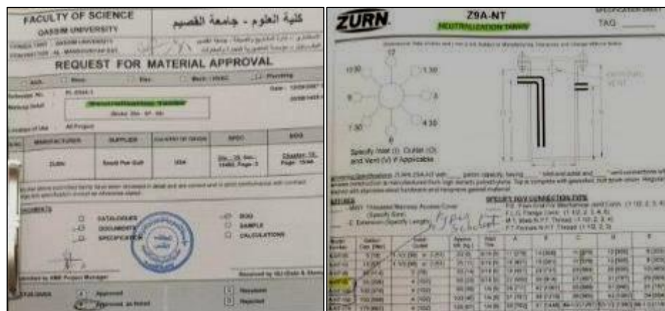
Figure 16. Copy of material submittal/ Request for material approval (Neutralization tanks) in Qassim University.
