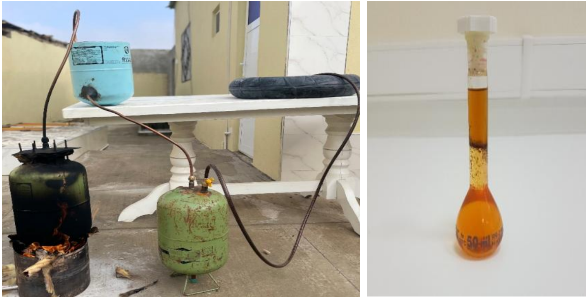
Figure 5. A process for converting plastic waste into a liquid fuel
