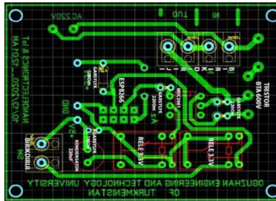
Figure 3. Smart lighting system board
