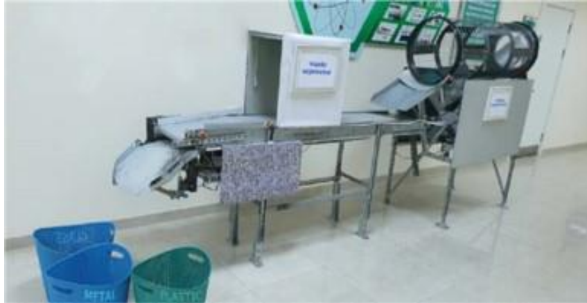
Figure 1. Automated waste sorting machine
