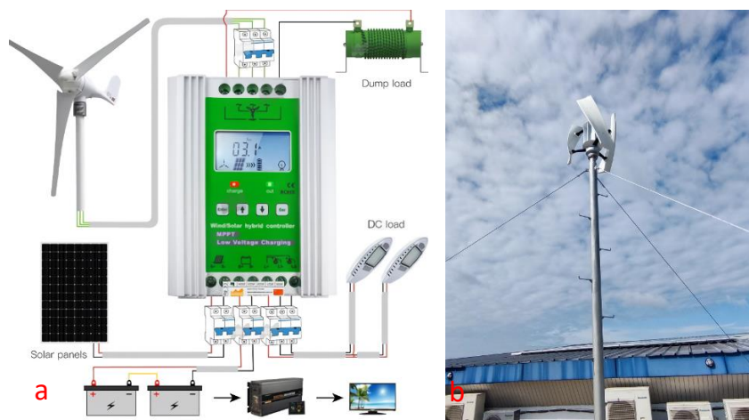
Figure 4. Pilot hybrid solar-wind power, (a) schematic, (b) wind turbine
