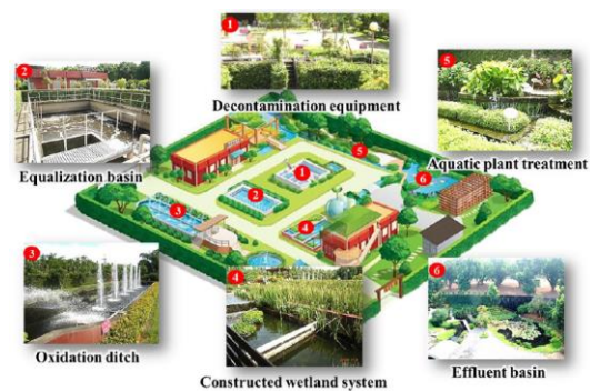
Figure 12. Domestic wastewater treatment process
