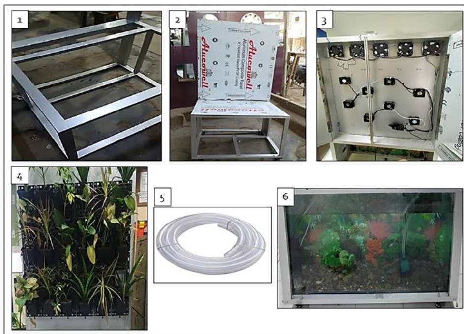
Figure 1. Fabrication phase (1) Bottom structure fame (2) Top cover of aluca bond sheet (3) Back view of fans placement at the top and center (4) Pots and plants (5) Irrigation pipe and (6) Aquarium and pump
