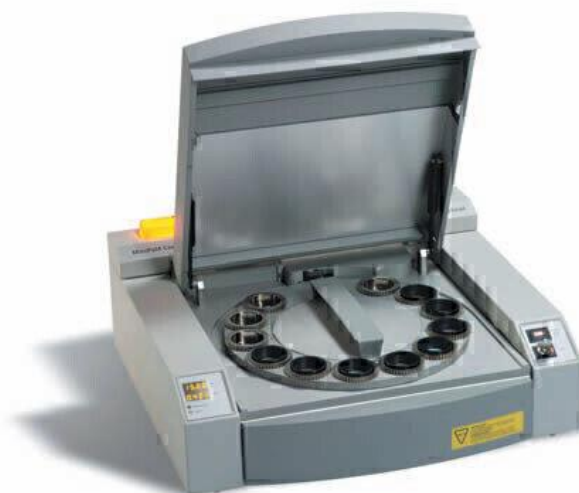
Gambar 2. Alat X-ray fluorescence spectrometer (EDXRF PANalytical Minipal 4)
