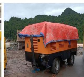
High pressure air compressor
