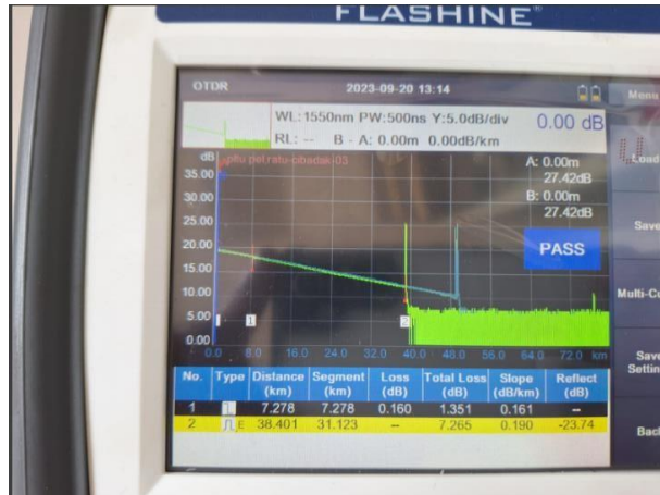
Gambar 2. Pengukuran redaman fiber optic
