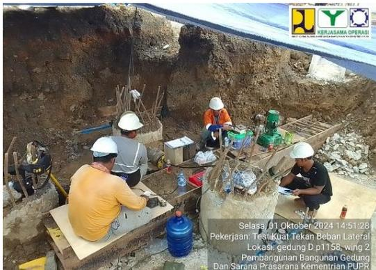
Gambar 15. Test beban lateral
