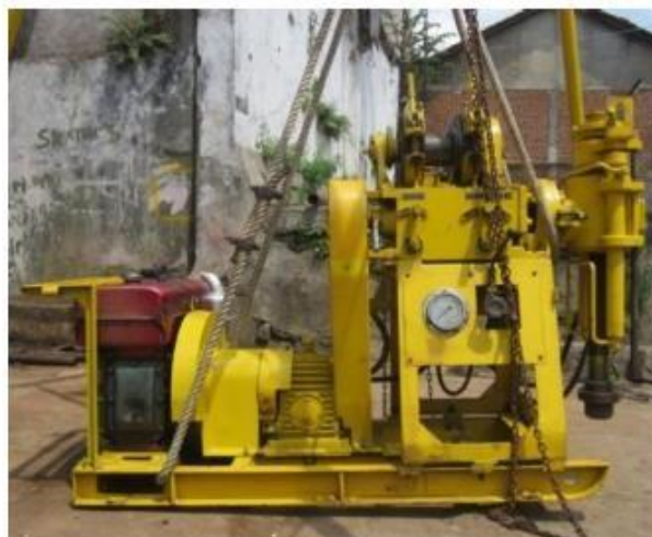
Gambar 1. Rotary boring machine (PT. MEC ReKayasa Indonesia, 2021)
