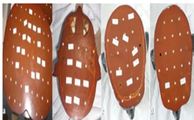
Figure 2. Position of TLDs in (a) lung, (b, c) brain and (d) eye lens phantom slices.
