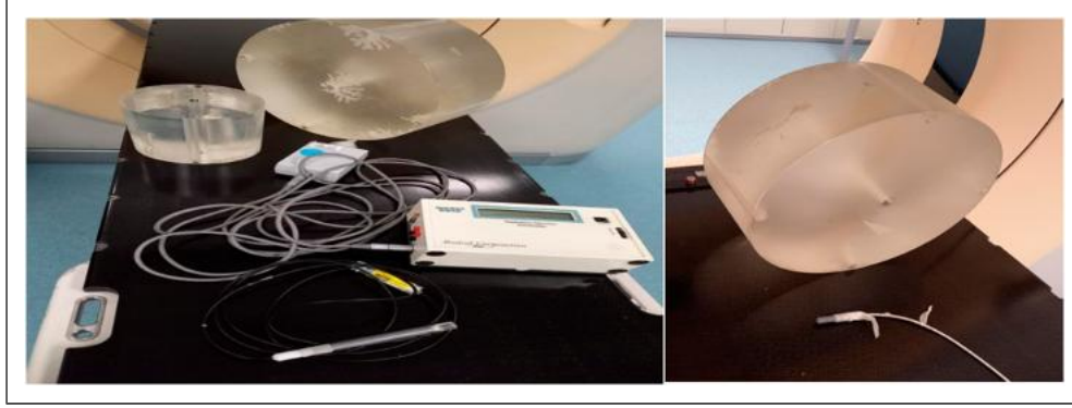
Figure 3. Set-up for CTDI determination.
