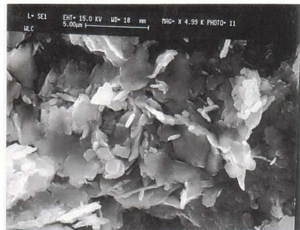
Figure 2. SEM photo of Clay in Pambik Village before firing
