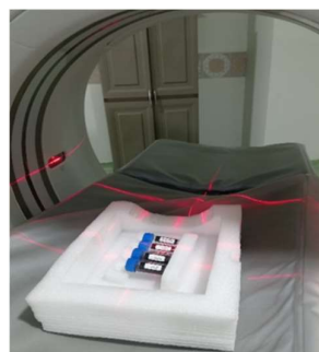
Fig. 2: Sample setup for CT scanning, showing the vials with Pt NPs in DIW, Pt NPs in 0.2% CMC, iodine solution, and a DIW control.
