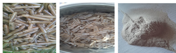
Fig. 1: Bamboo clam Ensis S.P (a) Whole Shell (b) clam Shell form (c) clam shell powder.
