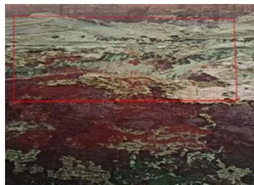
Fig. 6: Corrosion on the anode plate surface.
