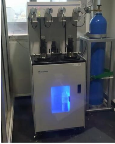
**Fig. 1:** Autopore V 9600 tools (documentation taken in LEMIGAS)
