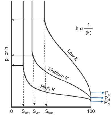
**Fig. 3:** Drainage Variation Curve with Absolute Permeability [12]
