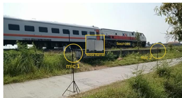
Fig 6. The positions for the Insertion Loss (IL) measurement at the existing scale
