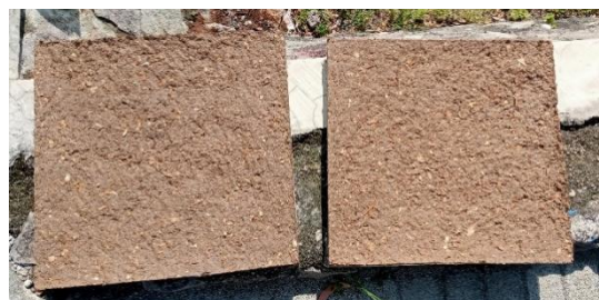
Fig 2. The dried blocks of the sustainable noise barrier
