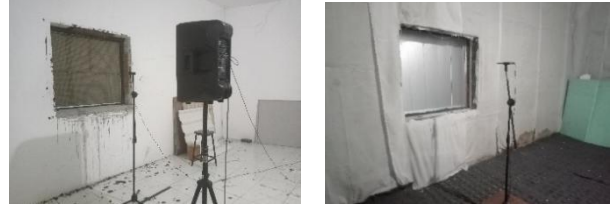
Fig 5. Measurement sound transmission loss (a) source position dan (b) receiver position
