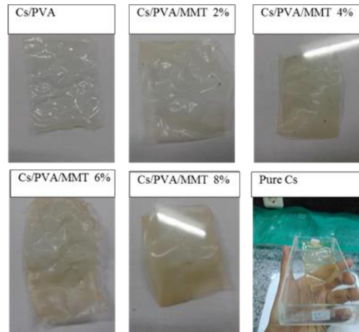
Figure 2 All membrane composites prepared by casting
