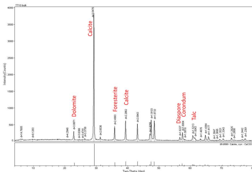
**Figure 5.** Selected XRD pattern (sample TT-10) showing the presence of diagenetic minerals (Dolomite) and metamorphic minerals (Forsterite and Diaspore) in the Limestone of Peneta Formation.
