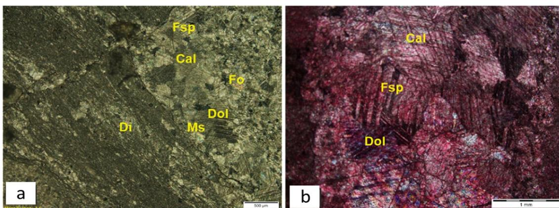
**Figure 3.** Photomicrographs from meta-mudstone facies on TT-08 (a) and TT-10 (b) samples show mudstone lithology. There are foliated structural features in sample TT-08 (a) and decussate texture in sample TT-10 (b). The mineral composition present includes carbonate minerals such as calcite (Ca) and dolomite (Dol) and accessory minerals such as muscovite (Ms), phlogopite (Phl), feldspar (Fsp), diaspore (Di), and forsterite (Fo).
