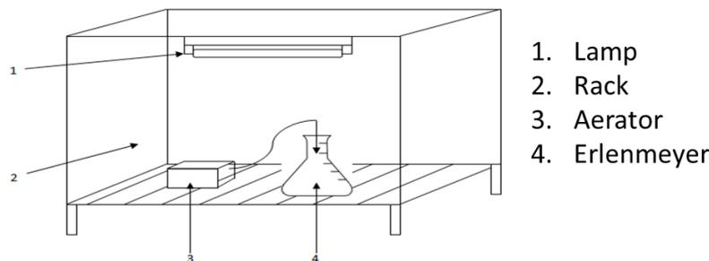
Figure 1. Experimental set-up of microalgae cultivation
