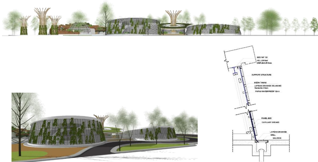
Figure 3.4. (a) Façade of building mass, (b) Greenwall of building mass, (c) Detail of greenwall
