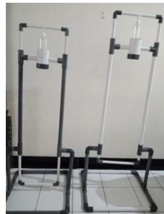
Gambar 3. Alat Hand Sanitizer Sistem Injak
