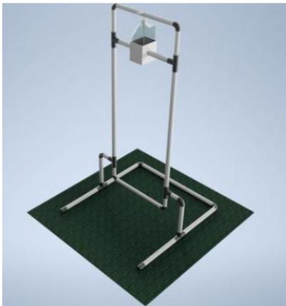
Gambar 2. Desain Alat Hand Sanitizer Sistem Injak
