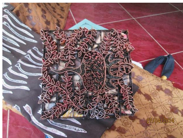
Gambar 3. Cap Canting Batik Mangrove
