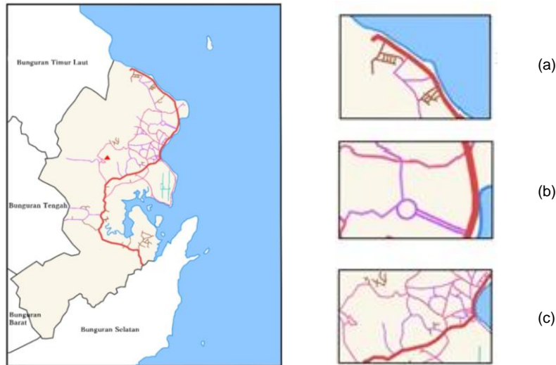
Figure 4. Road Pattern System Map of East Bunguran District, Ranai City. (a) Grid system. (b) Radial concentric system. (c) Irregular system.
