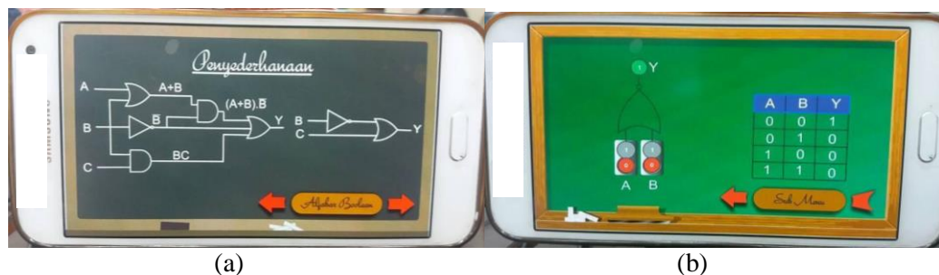
Figure 1. a).Logic simplification; b). NOR gate's interactive circuit
