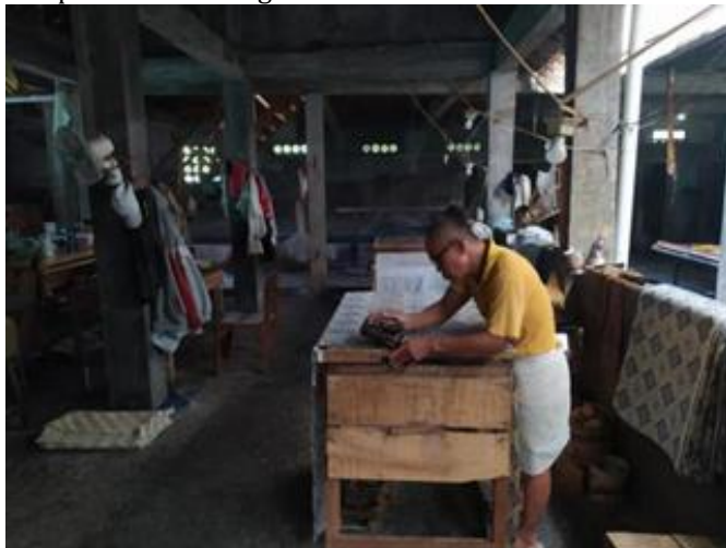
Figure 2. The coloring process using a batik stamp
