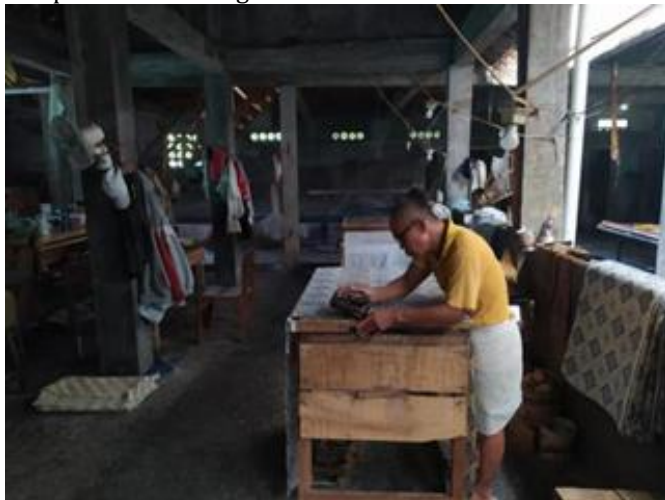
Figure 2. The coloring process using a batik stamp
