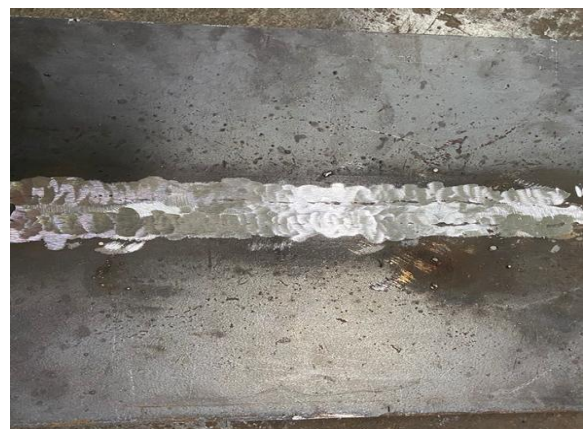
Fig. 8. Welding Results SMAW 100A
