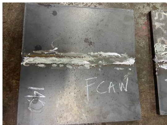
Fig. 6. Welding Results FCAW 140A
