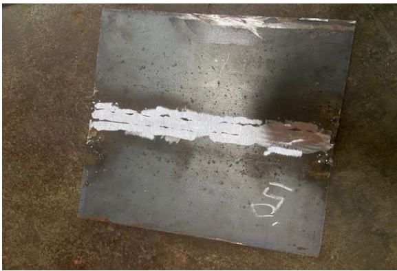
Fig. 9. Welding Results SMAW 120A
