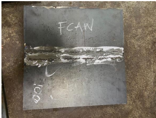
Fig. 4. Welding Results FCAW 100A
