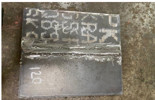
Fig. 5. Welding Results FCAW 120A
