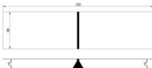
Fig. 2. Bending Test Dimension
