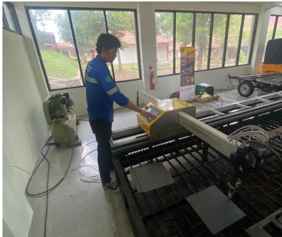
Fig. 10. Cutting Process with Cutting Machine
