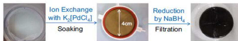
Figure 11. Prepared composite Pd / PES catalytic membrane [54]
