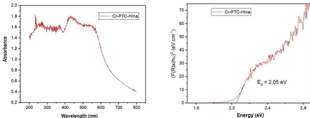
Figure 3. DRS-UV spectra and Tauc plot of Cr-PTC-HI<sub>n</sub>a-2.
