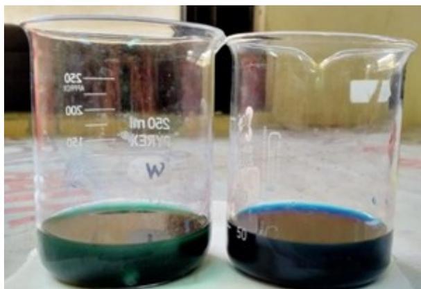
Figure 10. Methylene blue solution dispersed by Cr-PTC-HI<sub>na</sub> under alkaline conditions (pH 11) (left) and acidic solution (pH 2) (right).
