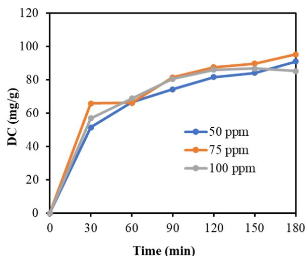
Figure 7. Degradation capacity Cr-PTC-HIna in various methylene blue initial concentration.
