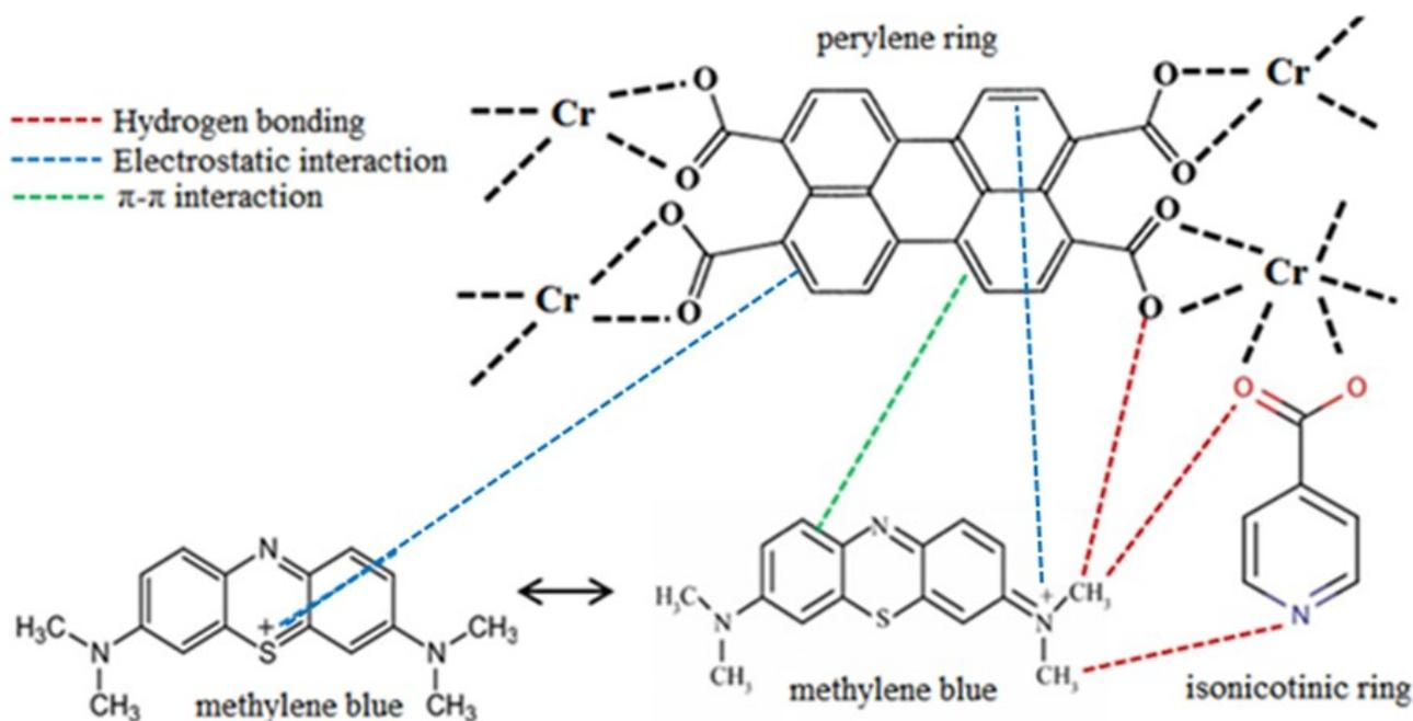
Figure 6. Possible interactions between methylene blue and Cr-PTC-HIna.
