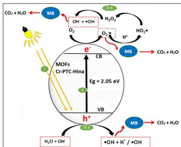
Figure 11. Photocatalytic methylene blue degradation mechanism by Cr-PTC-HI<sub>na</sub> under mercury lamp as visible light source.
