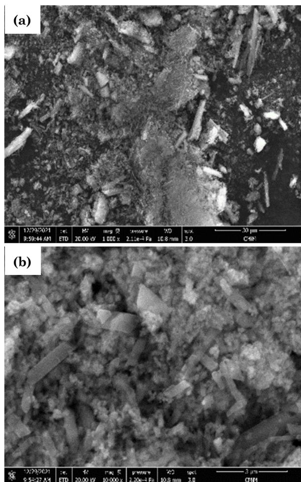
Figure 4. Morphology of Cr-PTC-HIna with (a) 1000x, and (b) 10000x magnification.
