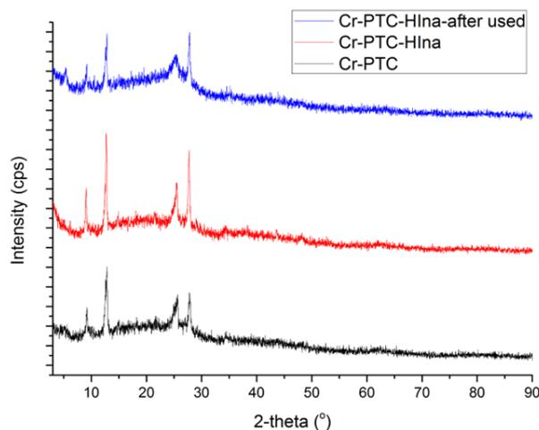
Figure 1. Diffractogram pattern of Cr-PTC and Cr-PTC-HIna (before and after used)
