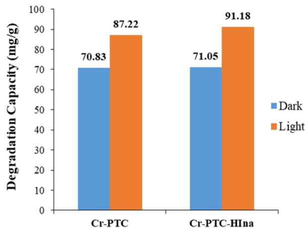
Figure 5. Degradation capacity of methylene blue by Cr-PTC and Cr-PTC-HIna.
