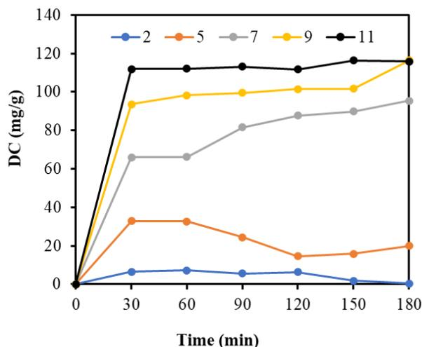
Figure 9. Degradation capacity of Cr-PTC-HI<sub>na</sub> in the variation of pH.
