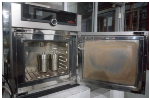
Figure 1. Hydrothermal reaction in stainless steel jacket and inner Teflon liner.
