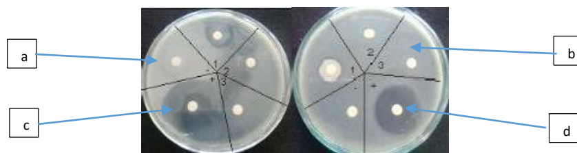
Figure 4.3 Results of Endophytic Bacteria Screening by Paper Disk Diffusion Method. Note: Bacterial cells (a) Staphylococcus aureus and (b) Staphylococcus epidermidis , (c) Disc paper, (d) Inhibited zones (1) Endophytic bacteria isolate code B23, (2) Endophytic bacteria isolate code B14, (3) Endophytic bacteria isolate code A2, (+) positive control of chloramphenicol, and (-) negative control.
